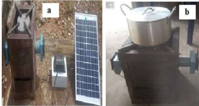
Figure 3: Developed flame sensor-controlled biomass stove and experimental setup (a) Complete experimental setup with solar panel and controller (b) Biomass stove with cooking pot
